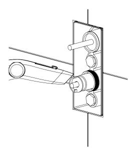
Attach the escutcheon pieces by screwing onto the threads on the valve body.
